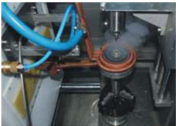
Fig. 1 Contour ISH of gear wheels system
