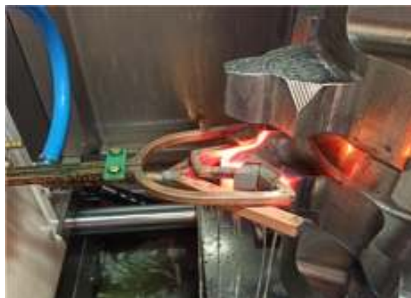
Fig. 2 Tooth-by-tooth ISH system
